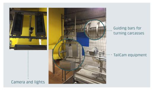
Figure 1: TailCam system.
