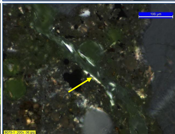
Monosulphate phases are occasionally observed in the crack. X-polarised light.
