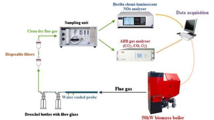
• By Measurements  $NO_x$  is normally found in the range 100-250ppm, dependent on the wood pellet (biomass) and combustion temperature
