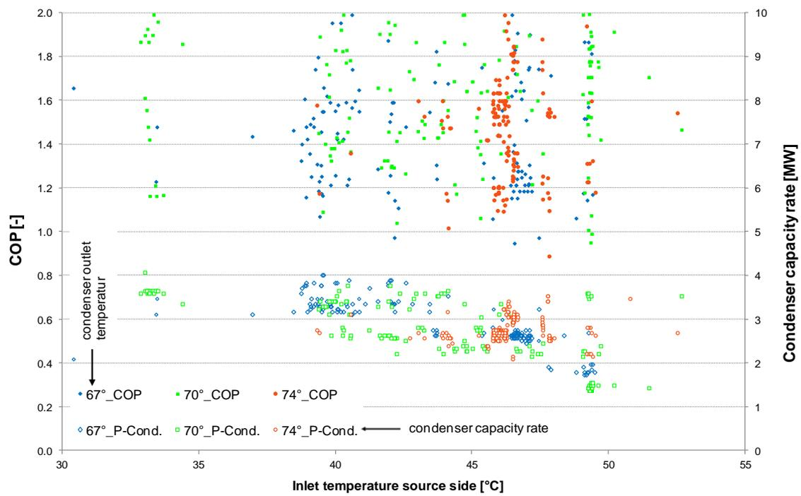
**Fig. 26:** Heat pump performance map based on 10-minute values from 2014.
