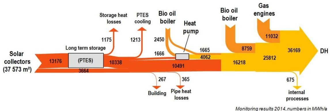
**Fig. 17:** Energy flow diagram according to 2014 monitoring data.
