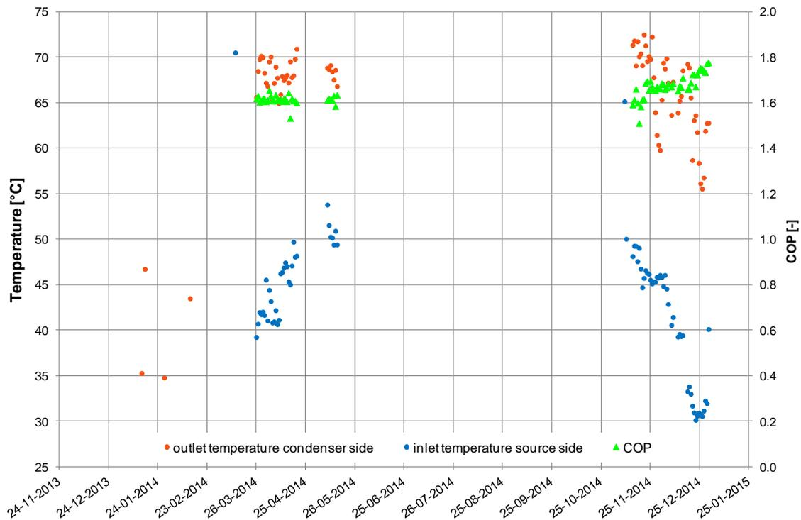
**Fig. 25:** Heat pump operation conditions in 2014 (daily mean values).
