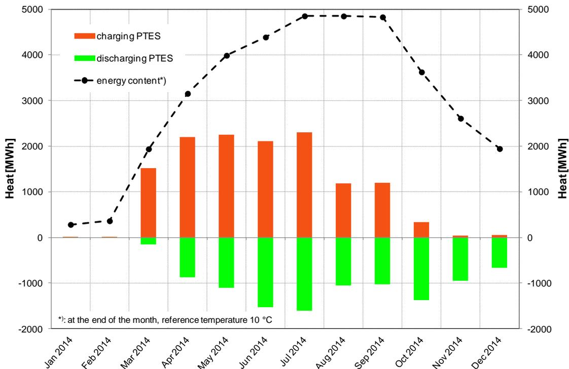
**Fig. 21:** PTES monthly heat balance according to 2014 monitoring data.
