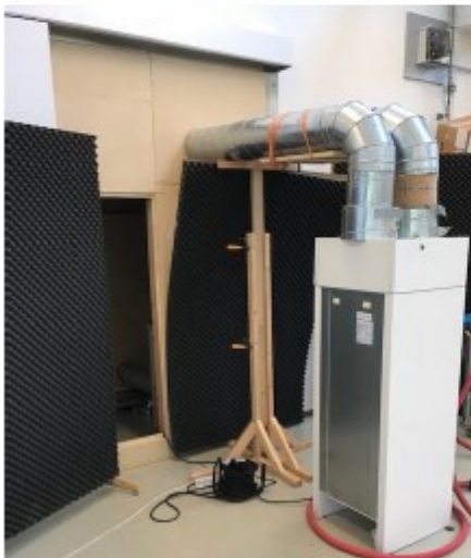
Figure 2: Sound power from duct, mounted flush in wall. Based on measurements of sound pressure in reverberant room using ISO/EN 3743-1.
