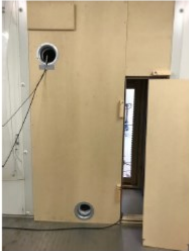
Figure 1: Sound power from the surface of the unit measured as ISO/EN 9614-2. Sound intensity measurements on eight surfaces, each with an area of 1 m 2 . The sound absorbing screens behind the unit improve the acoustical conditions.
