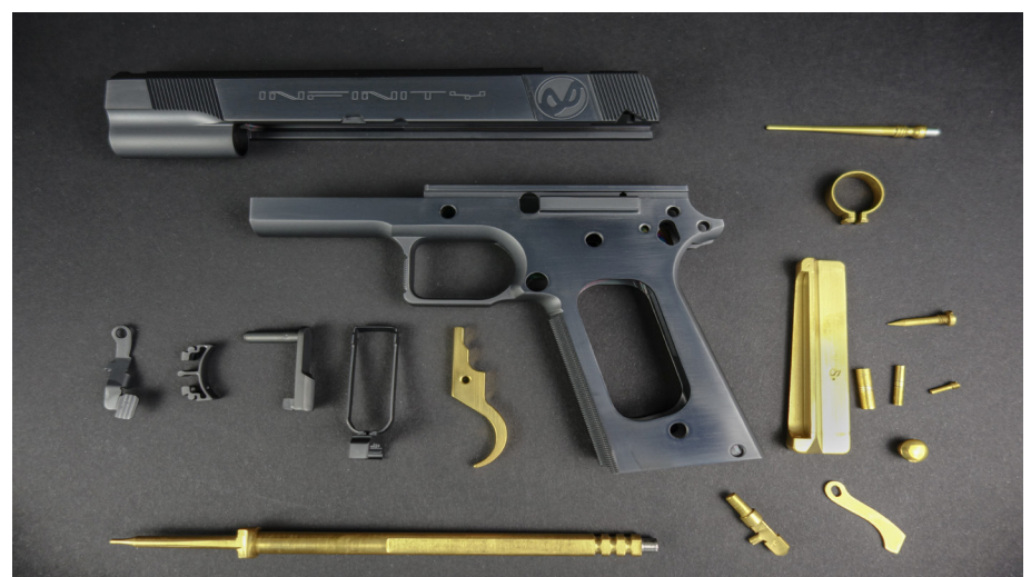
Pistol parts from the company "INFINITY" coated with TiN and DLC-TR for both functional and decorative purposes.
