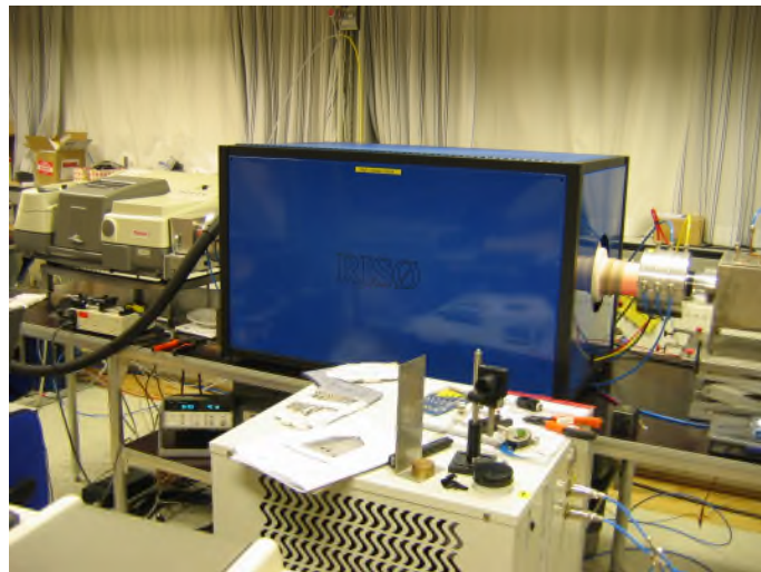
Hot gas cell DTU Temperature range: 23 °C - 1600°C UV, VIS, IR, FAR,...
