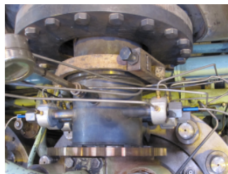
Hot gas cell DTU Temperature range: 23 °C - 1600°C UV, VIS, IR, FAR,...
