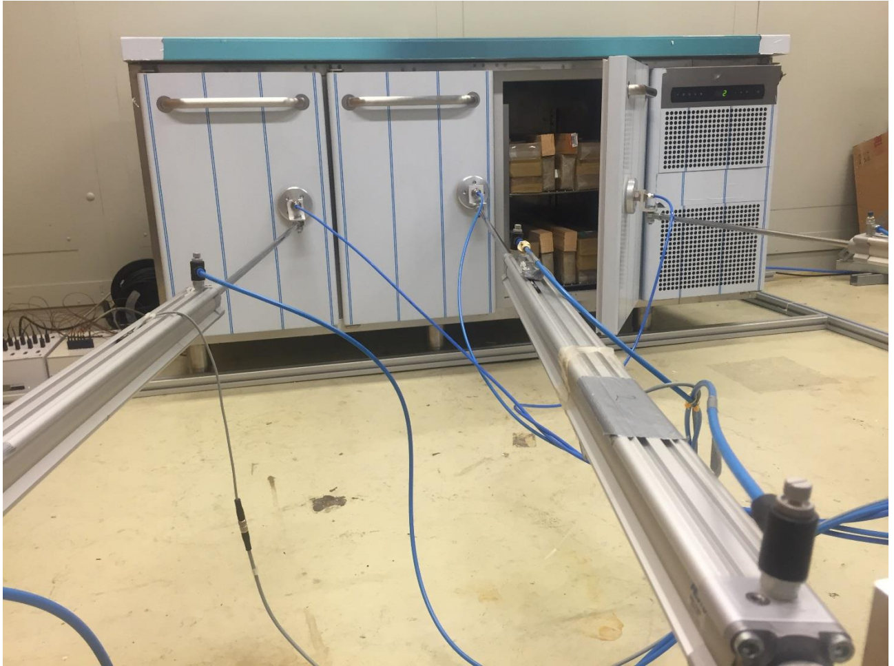
Figure 1: Photo of the test facility for the refrigerated counters under study. The basis of the project is a three-door counter. The three robot arms are opening the doors according to EN16825 (2016).
