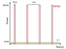
Figure 1: The power output as a function of time. The green line illustrates the constant power (10 kW) applied in a DC process. In contrast, the power in a HiPIMS deposition is significantly higher, but only in short bursts.
