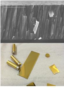
Figure 2: Top: Cross-sectional SEM image of the new TiN-HP-LT coating deposited on a Si substrate. The scale bar is 500 nm. Bottom: Test samples coated with the new TiN-HP-LT coating.
