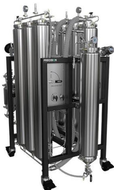
**Figure 12.** An example of a closed-loop hydrocarbon extractor. This extractor features individual control of solvent, vacuum, nitrogen, and venting via centralized instrumentation panel for ease of operation. This equipment is C1D1 Compliant & Designed for GMP integration with PSI Certified for 50 State Compliant. This XMU Hydrocarbon extractor model can process up to 100 kg per day shift.<sup>56</sup>
