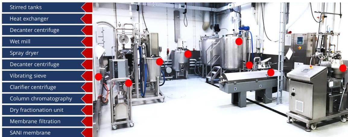
**Figure 1.** Generic cascading unit operations for upcycling plant biomass utilized in the ProEnrich project.
