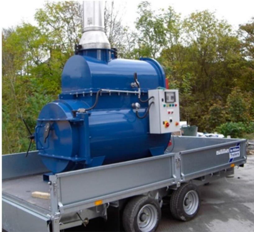
**Figure 17.** The Matthews Environmental Solutions mobile incinerator. The incinerator is fitted, along with a generator and fuel tank on to a flatbed trailer. To speed up start-up preparation time, the incinerator incorporates a hinged chimney to enable it to lie horizontally during transportation.<sup>73</sup>
