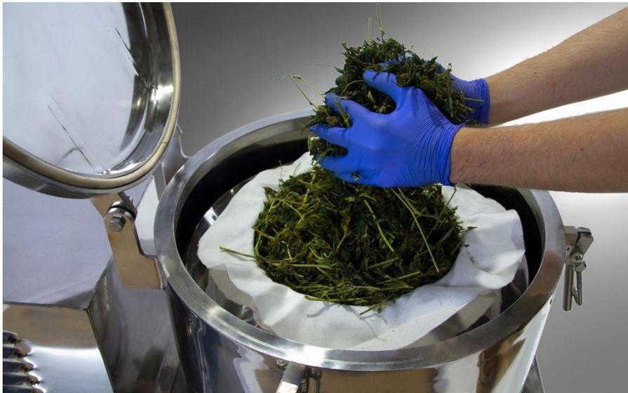
**Figure 13.** Loading of the cannabis plant material into a Pilot-scale extraction vessel. The ethanol is supplied in the vessel either through shower or flooding inside the vessel.<sup>58</sup>
