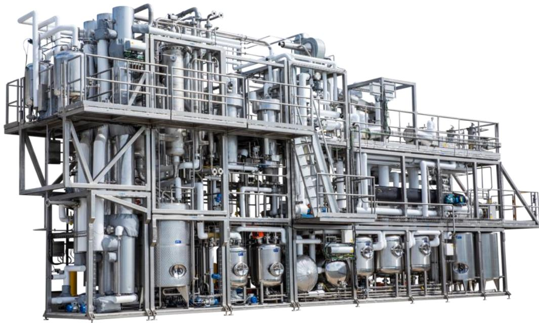
**Figure 14.** Precision KPD Series: Vulcan - Industrial Cannabis Extraction Plant. This is a close-loop extraction facility where the feed material (i.e. dried cannabis) is soaked in the ethanol, then subjected to a cold press to separate the extract and the solid residue. The ethanolic extract is then filtered and evaporated/ distilled to recover a concentrated cannabis-ethanol extract.<sup>21</sup>
