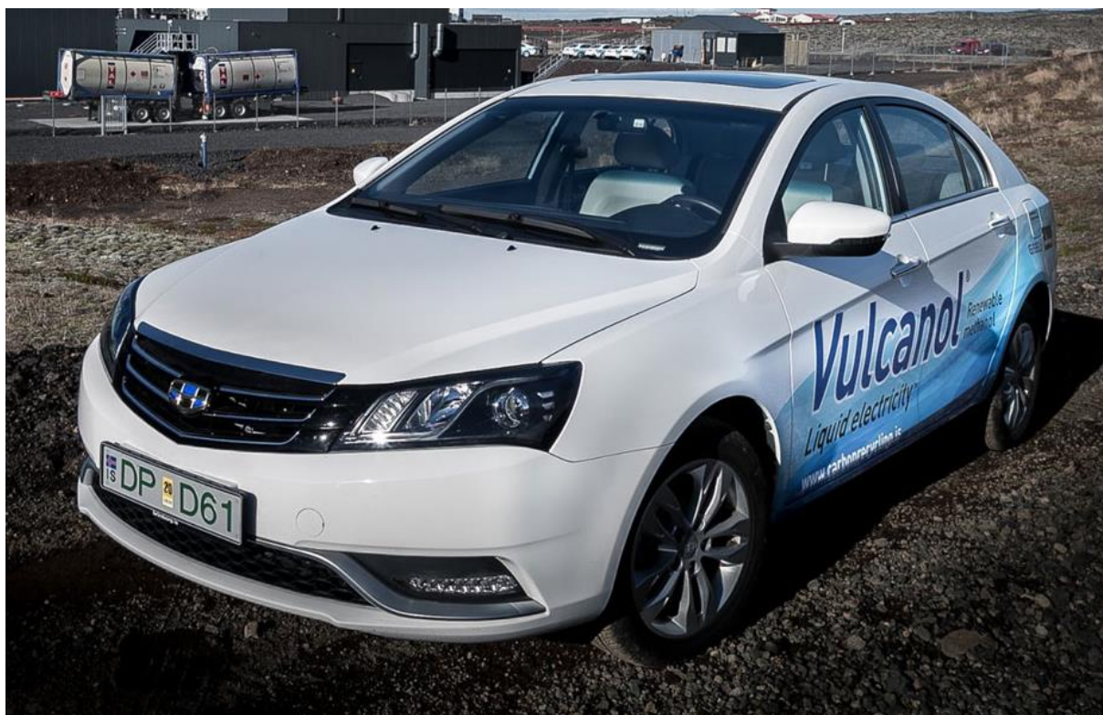
Figure 21 Geely Emgrand 7 with and engine for 100% methanol
