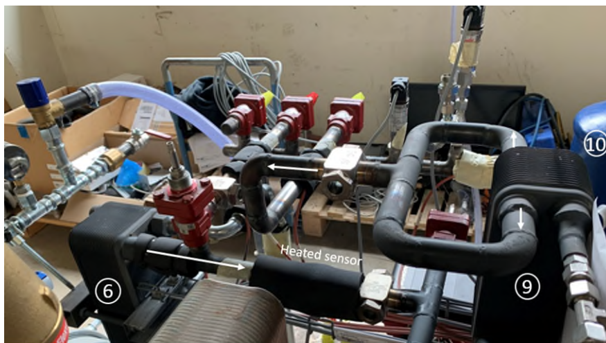
Figure 45: Heated sensor test setup. 6) Evaporator, 9) SGHX, 10) Suction accumulator.
