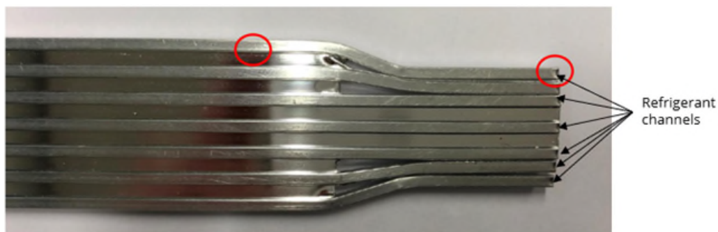
Figure 52: Micro channel WEB-MPE profile.
