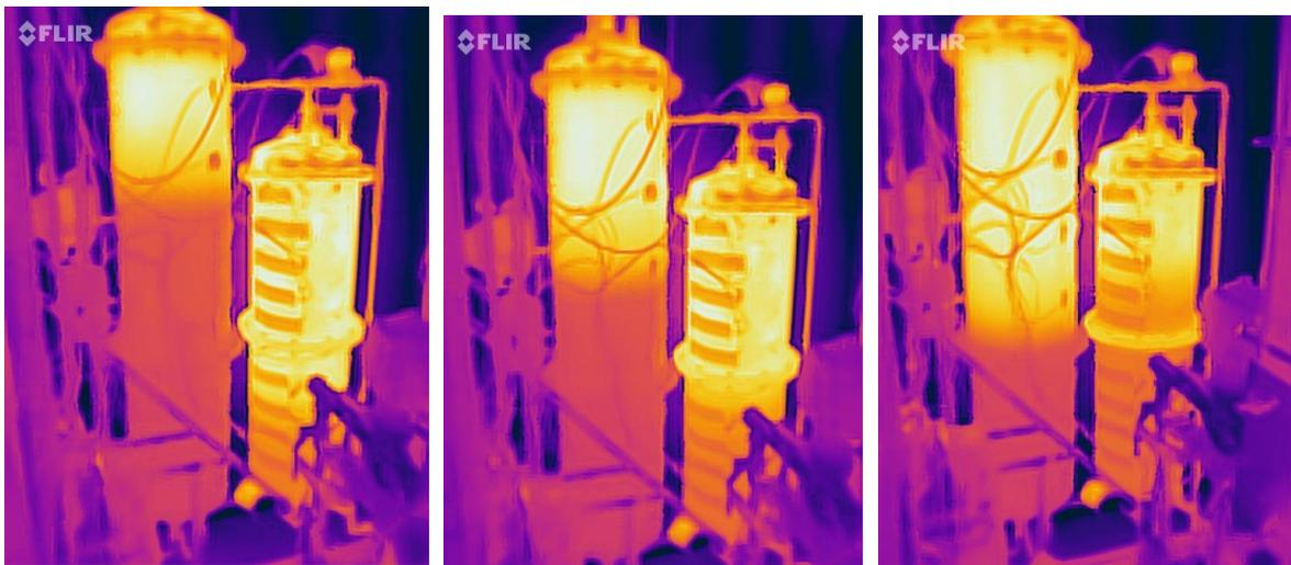
Figure A3.2: Development of temperature profiles in buffer and charge tank. The charging process is being continued. For both tanks, the upper part is warm, and the lower part is cold.
