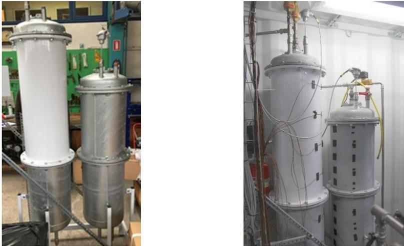
Figure 42: Left: Buffer tank and charge tank. Right: Tanks with sensors mounted.
