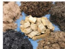
Figure 1. Wood substrate components vary in their manufacturing processes, particle size and shape, and color, as well as the ability to be easily mixed.
