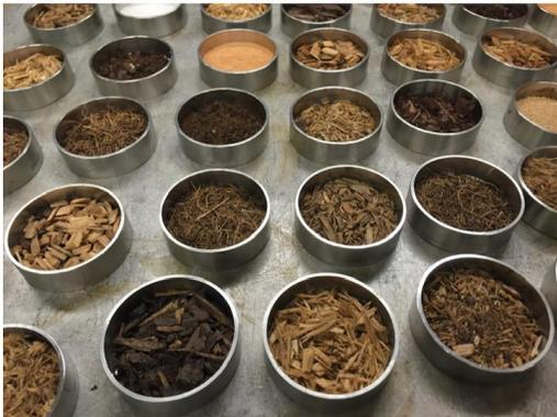
Samples of soilless substrate materials to be tested for physical, chemical, hydrological and biological properties in the North Carolina State University research lab. Brian E. Jackson
