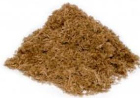
To support environmentally-friendly horticulture, we developed TIMPOR®. TIMPOR® is a specially processed structural wood fibre used as a peat substitute, allowing us to reduce the amount of peat used in our products or remove it completely.
