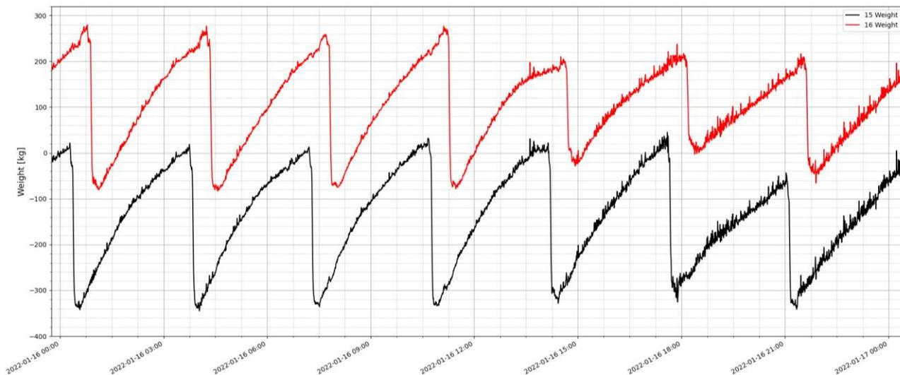
Figure 14: Weight measurements of evaporator #15 and #16 at Brædstrup
