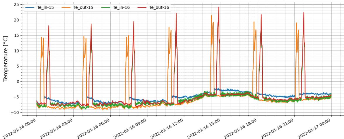
**Figure 12: Measurements of evaporation temperatures at inlet and outlet headers on evaporator #15 and #16 at Brædstrup**
