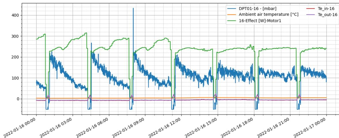
**Figure 13: Measurements of differential pressure between inlet and outlet tubes on the ammonia side for evaporator #16 at Brødstrup**
