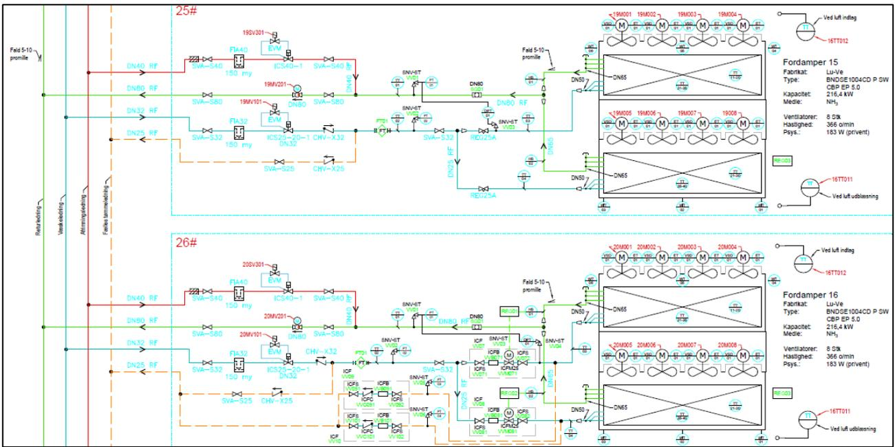
Figure 7: PI-diagram of evaporator #15 and #16 at Brødstrup Fjernvarme
