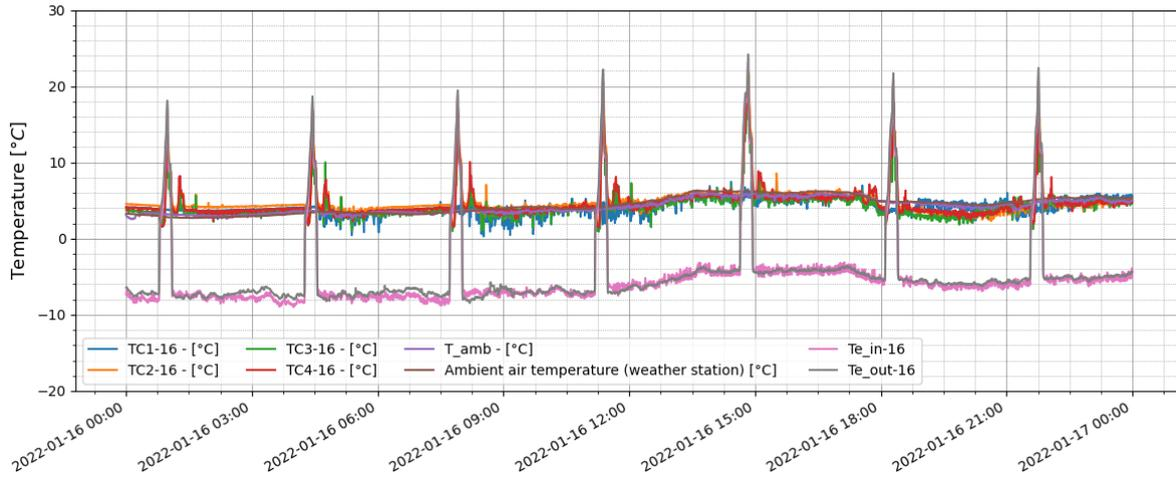
**Figure 10: Measurements of the inlet temperatures for the ambient air underneath evaporator #16 at Brødstrup**
