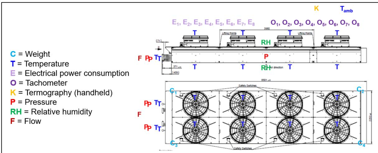
Figure 8: Specification of various measurements on evaporator #16 at Brødstrup Fjernvarme
