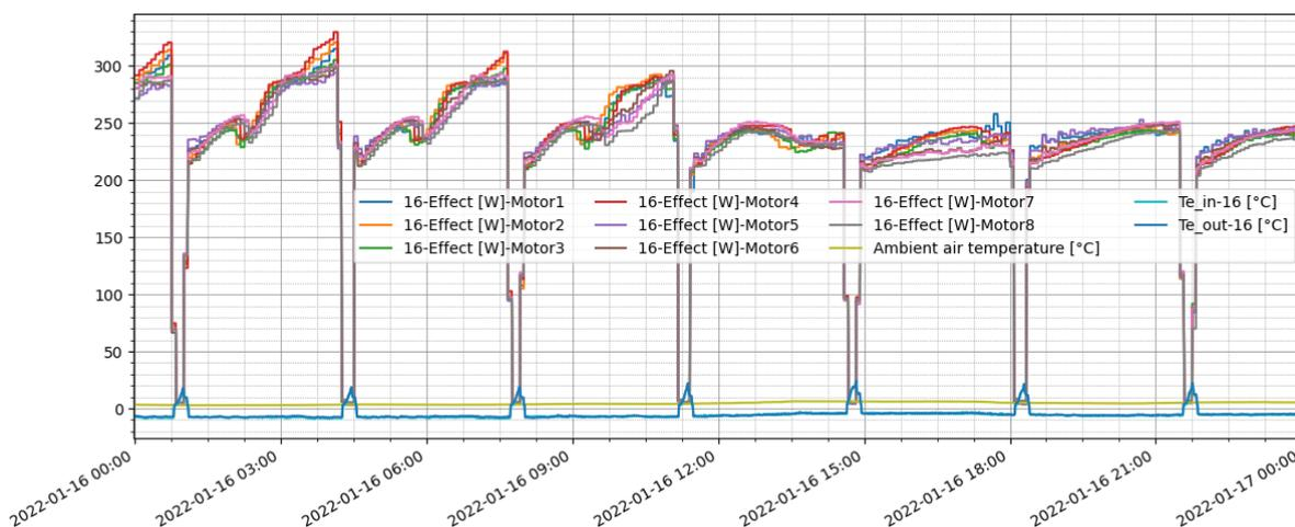
**Figure 11: Measurements of electrical power consumption for the eight fans on evaporator #16 at Brødstrup**
