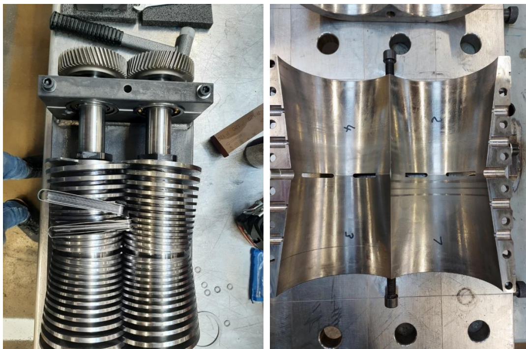
Figure 25: Setting the gap between the spindles to adjust the gears for synchronous rotation (left), one half of the housing insert with water injection ports for left and right spindle assembly (right).
