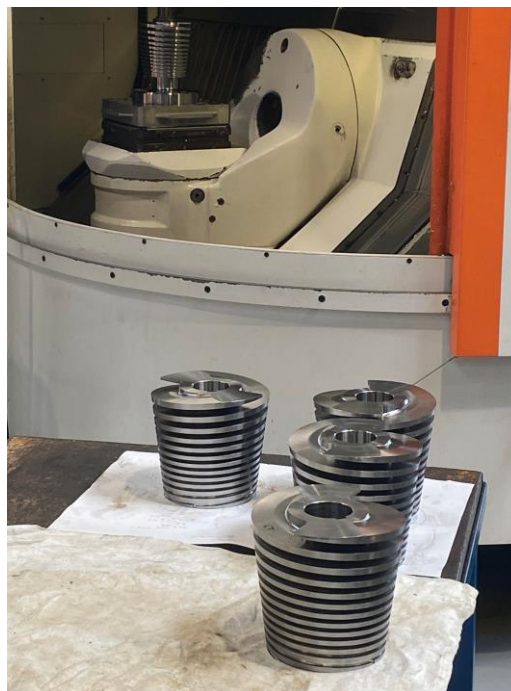
Figure 21: The conical spindles manufactured by 5-axis machining at CS Techcom.
