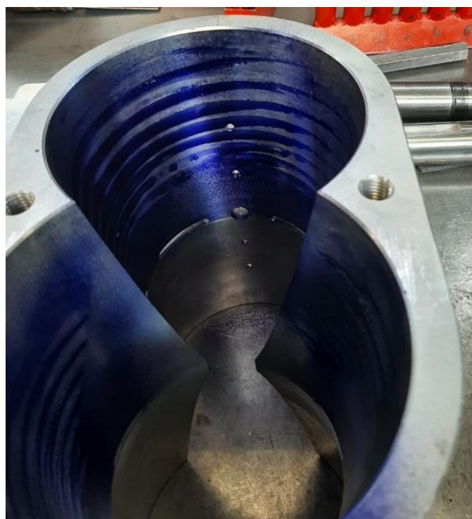
Figure 22: The conical bore inside the housing insert, painted to check the gap to the spindles
