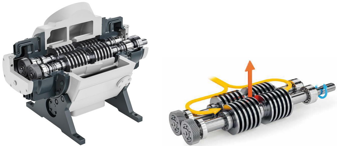
Figure 15: KRAL water pump, Z series, with symmetric, double intake to eliminate axial forces.
