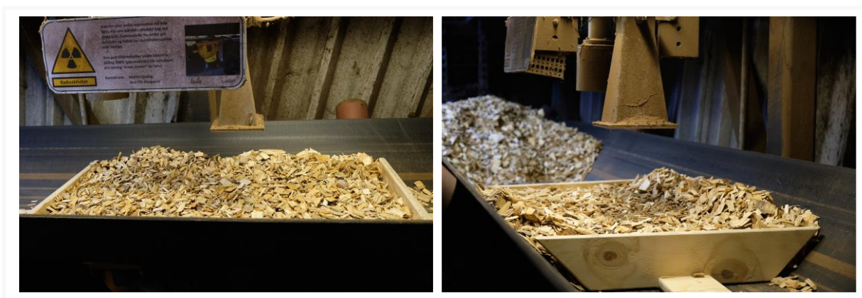
Figure 4. Sample material place at the conveyor belt at VERDO's CPH plant for the test measurements using the MW system. The sample material was prepared in advance at DTI, as described in the text.
