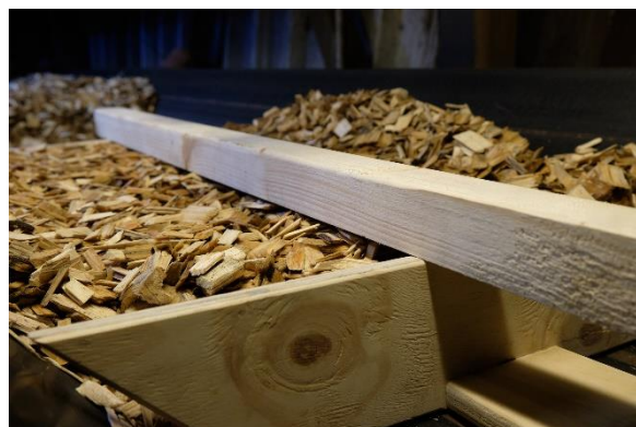
Figure 5. The woodchip test material is carefully level, to secure a constant layer thickness.
