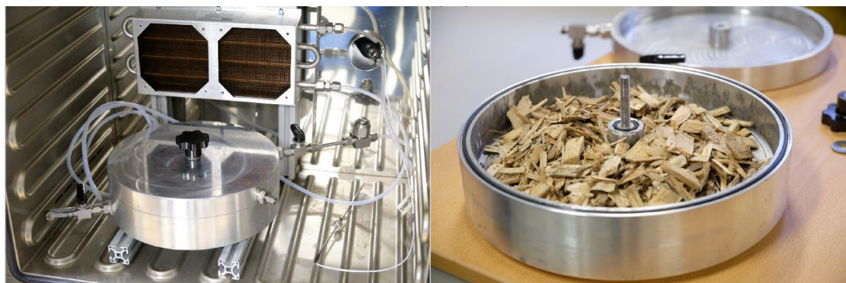
Figure 6. The setup for reference water-content measurement at DTI. Left: The heated sample chamber; Right: A sample being placed in the chamber.
