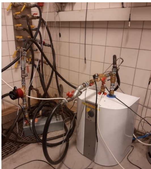
Figure 7 EI-booster with circulation of domestic hot water.
