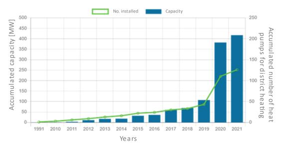
Figure 25. Overview of large-scale heat pumps for the Danish district heating network [4].
