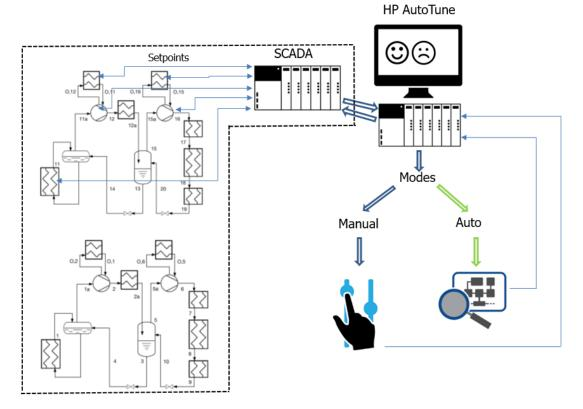
Figure 2 – Concept for HP AutoTune.
