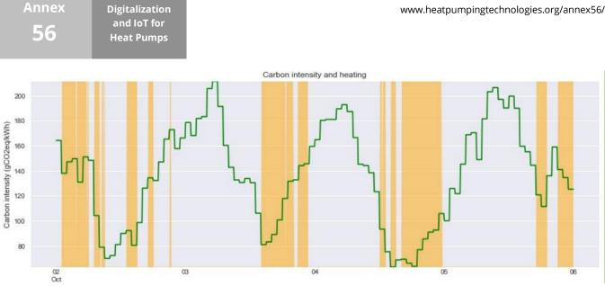
Figure 2: Predicted carbon intensity (green) and periods at which the heat pump is turned on (orange). The installation is located in Denmark.
