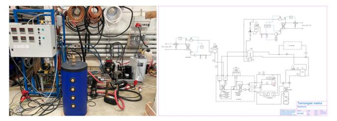
Figure 2: Preliminary test setup with the multi-source heat pump at Danish Technological institute.
