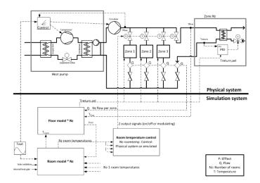
Figure 4: Physical and simulation system.
