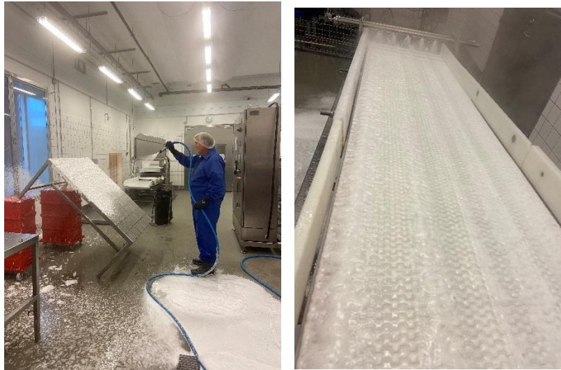
Figure 3. Manual cleaning of steel surfaces and cleaning of conveyor belt using a spray bar.
