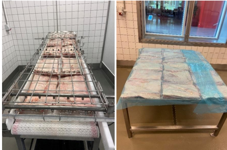
Figure 1. The surfaces were soiled with meat/bacteria for approx. 18 hours to simulate a normal production day in the meat industry.
