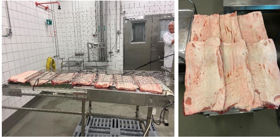
Figure 1. Soiling of surfaces with meat inoculated with \sim 4.5-5.5 \log \text{cfu}/\text{cm}^2 . The surfaces were soiled for approx. 18 hours to simulate a normal production day in the meat industry.
