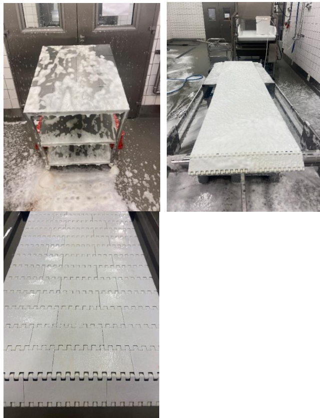
Figure 3. Pictures of surfaces with soap (10 min after application) and the belt after cleaning and disinfection.
