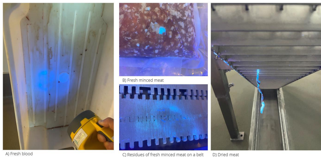
Figure 4. UV- inspection of fresh meat and blood (a,b,c) and dries meat (d).
