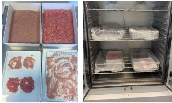
Figure 2. Soiled surfaces with meat suspensions inoculated with bacterial spoilers. All surfaces were incubated for 11 days for biofilm formation.
