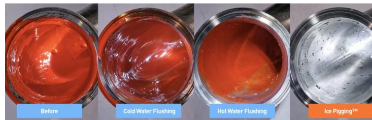
Figure 1. The cleaning effect of ice pigging compared to the use of hot or cold water.
