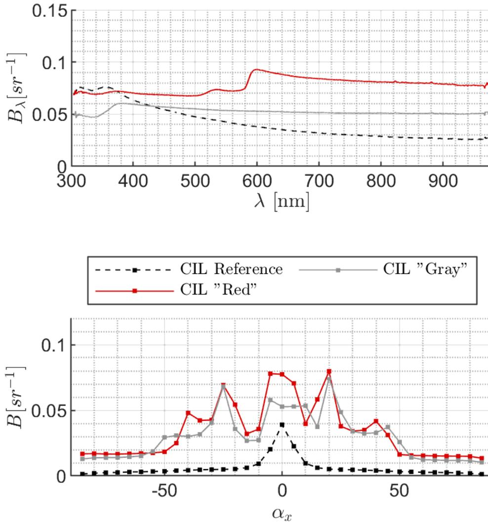
Figure 14: Spectral BRDF at  $\alpha_x = \theta = 0^\circ$  (top), total BRDF at  $\theta = 0^\circ$  (bottom) for CIL samples.
