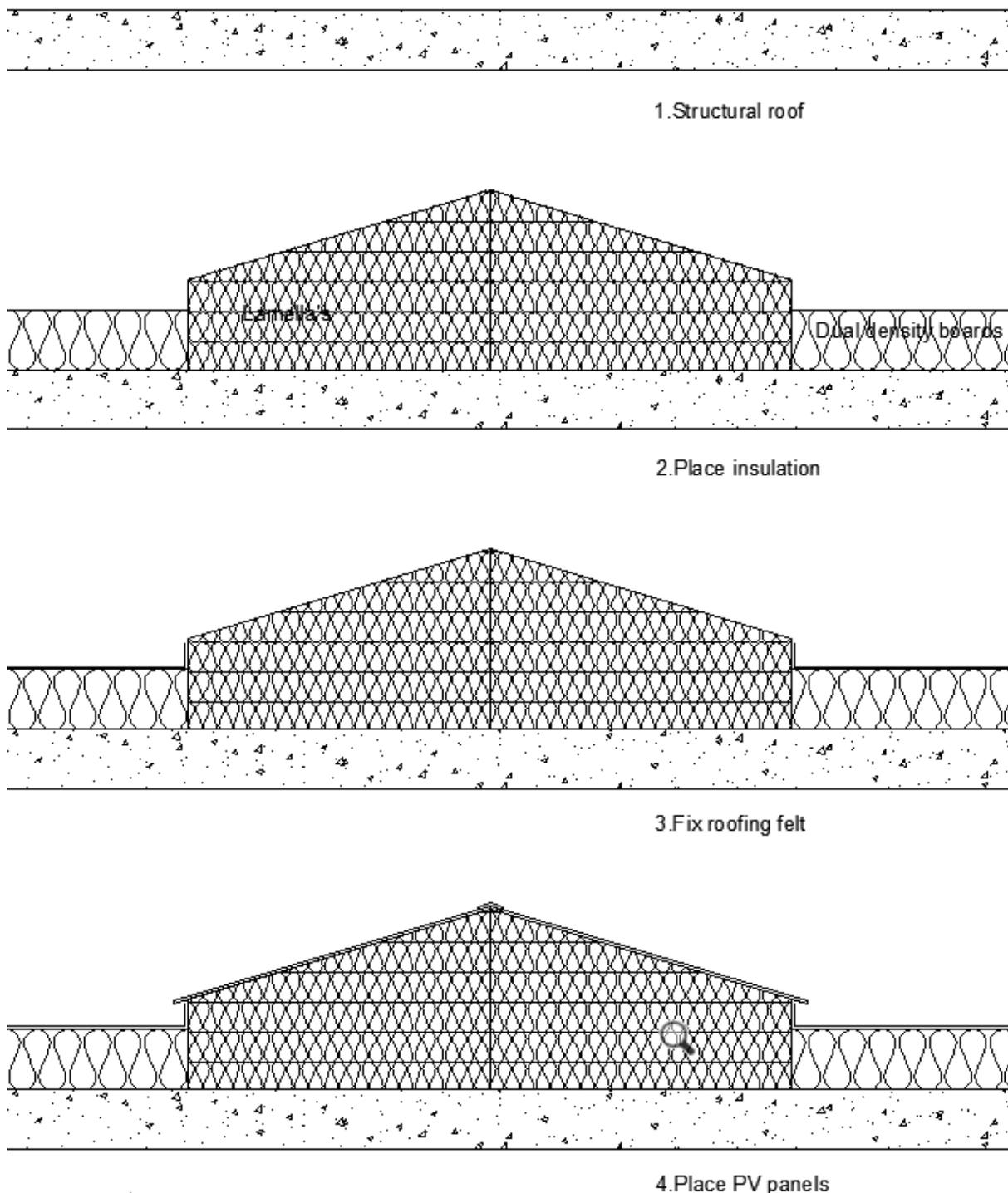
Figure 2: Final solution for a flat roof concept combining PV and insulation.
