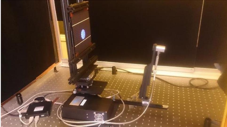
Figure 9: Photo of experimental BRDF setup.
