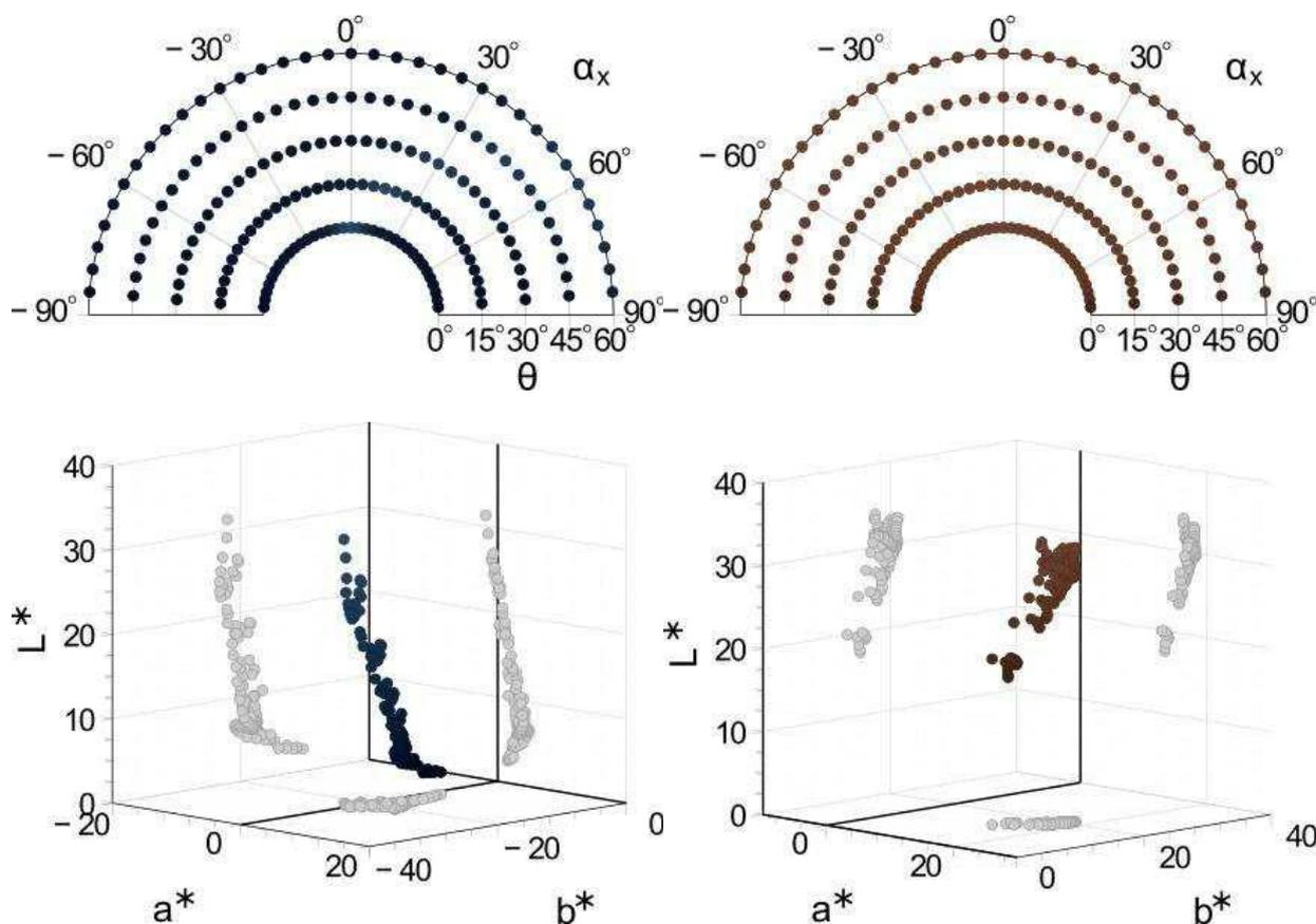
Figure 16: PCI "Blue" (left) and PCI "Terracotta" (right) in angular color representation and CIELAB color space.
