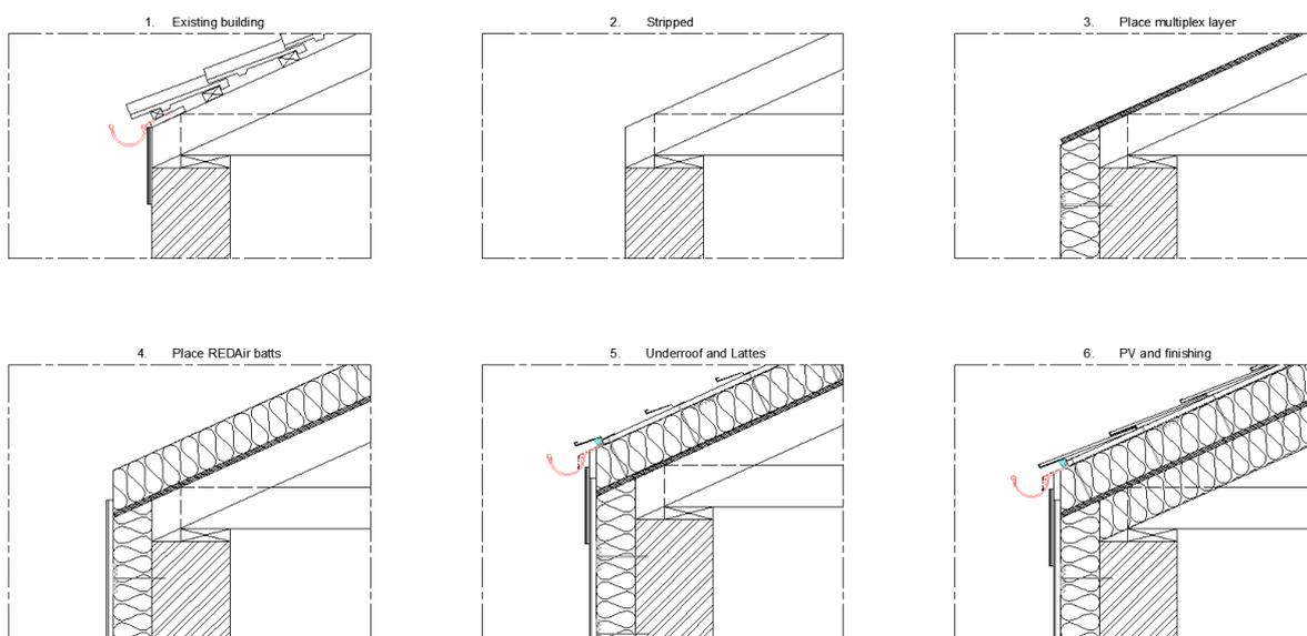
Figure 3: Final solution for sloped roof solution based on Rockwool's REDAir facade insulation system.
