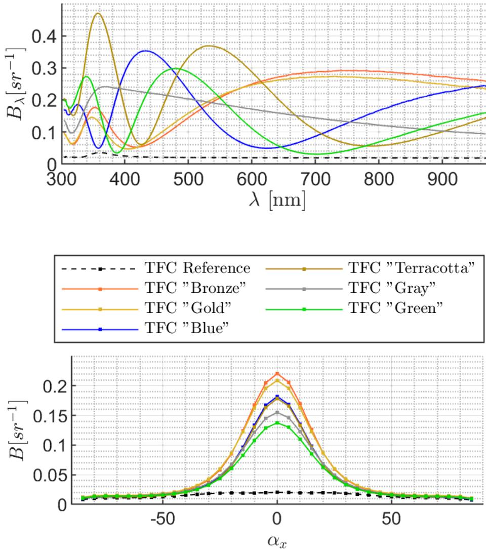
Figure 13: Spectral BRDF at  $\alpha_x = \theta = 0^\circ$  (top), total BRDF at  $\theta = 0^\circ$  (bottom).
