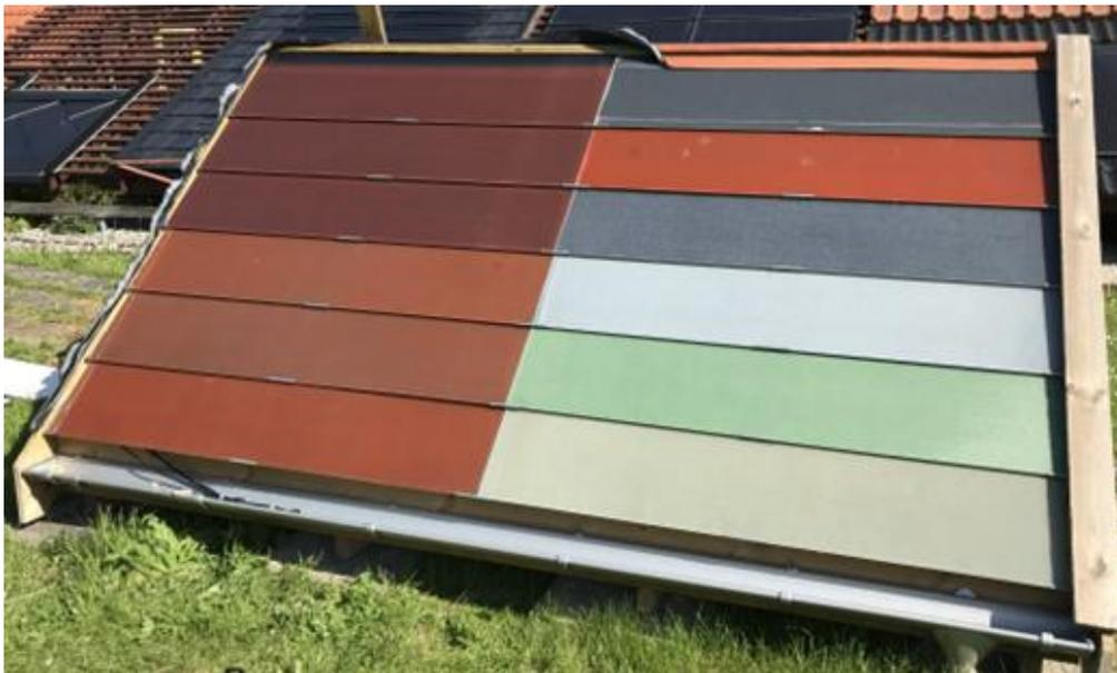
Figure 1: Photo of one of the experimental mockups showing different PV colors.
