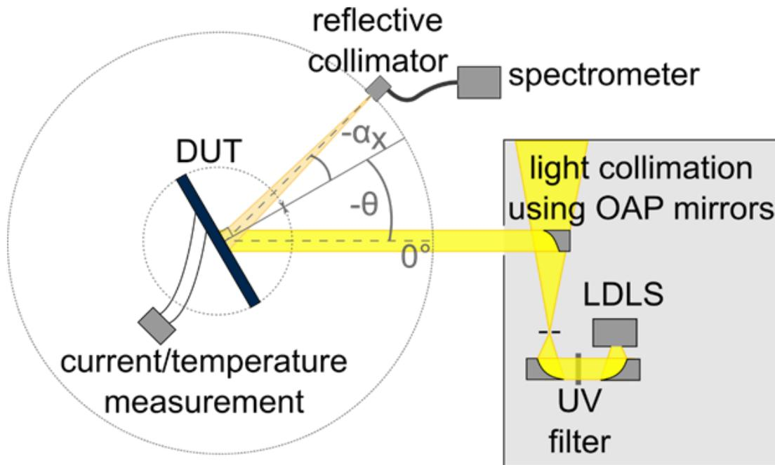
Figure 8: Schematics of experimental measurement setup for single-plane spectral BRDF:  $\alpha_x$  denotes the view angle, and  $\theta$  denotes the incidence angle of light.
