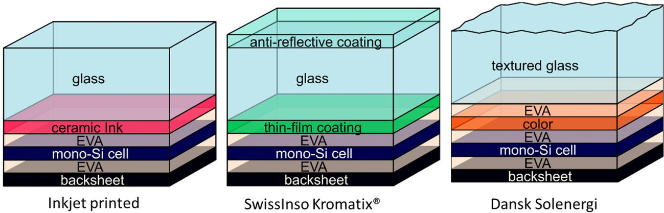
Figure 11: Conceptual drawings of the different colored technologies measured in the setup.
