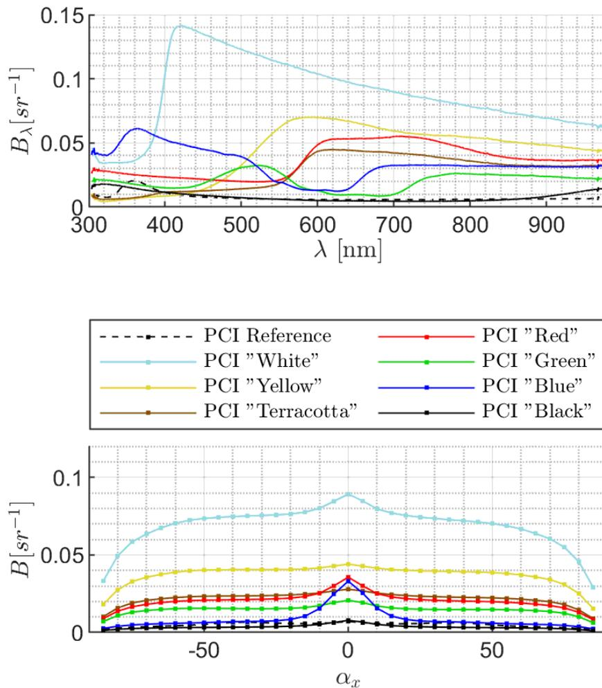
Figure 12: Spectral BRDF at  $\alpha_x = \theta = 0^\circ$  (top), total BRDF at  $\theta = 0^\circ$  (bottom) for PCI samples.
