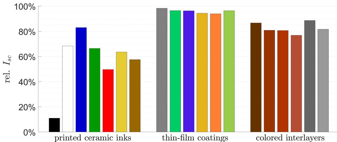
Figure 23: Short circuit measurements relative to a non-colored one cell PV module.
