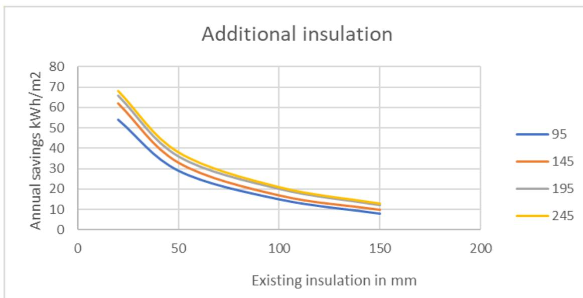
Figure 7 Annual savings for added insulation of the roof
