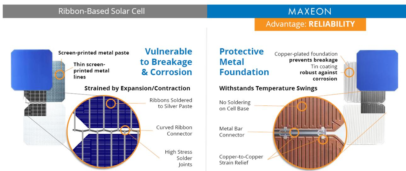
Figure 25: Advantages of the back-contacted cells according to Maxeon
