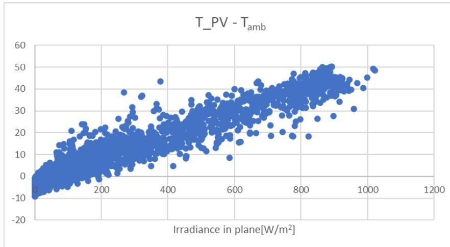
Figure 30: Measured correlation between panel overtemperature and solar intensity.
