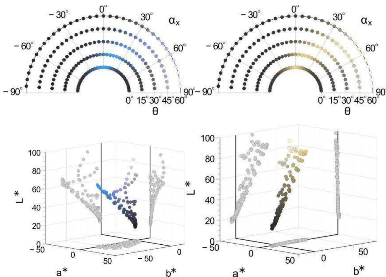
Figure 18: TFC “Blue” (left) and TFC “Gold” (right) in angular color representation and CIELAB color space.
