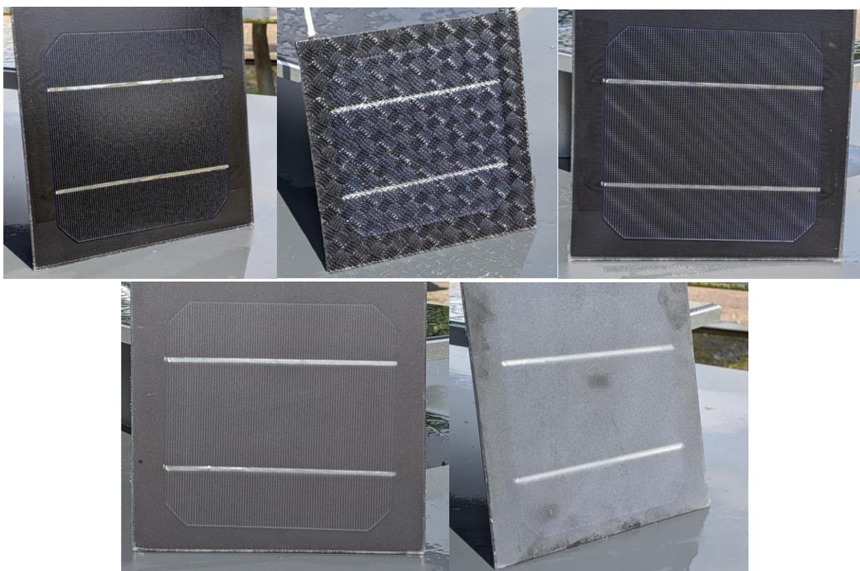
Figure 24: Visual comparison of different glass types: Reference, textured1, textured2, etched, sand blasted.
