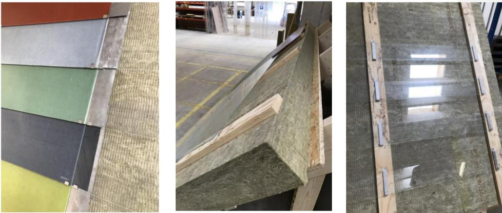
The PV elements are hung inside hooks that are in turn screwed to lattes. Installations of the PV panel are easier in this manner.
