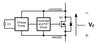
"Smart Diode" TO-263-3 and function diagram.
