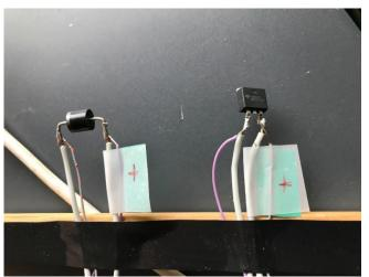
Figure 1 Diodes in free air connected with power and sense wires.
