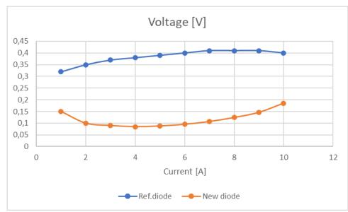
The voltage drop over the sense wires shows very different behavior for the two types:
