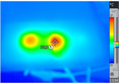
Figure 7 Thermal image from the glass side. Now the standard diode is warming the glass via the thermally conductive filler. The temperature rise of the active diode to the right is hardly seen compared to the others.
