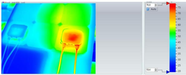
Figure 9 Temperature on the back immediately after removing insulation.
