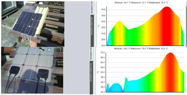
Figure 10 Temperature profile across the two junction boxes from front and rear.
