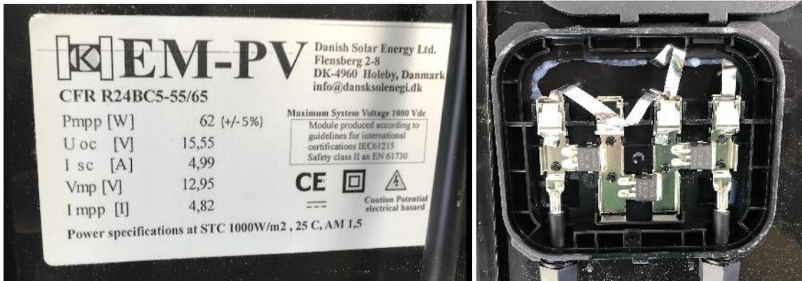
Figure 12 Name plate and junction box of the new modules.
