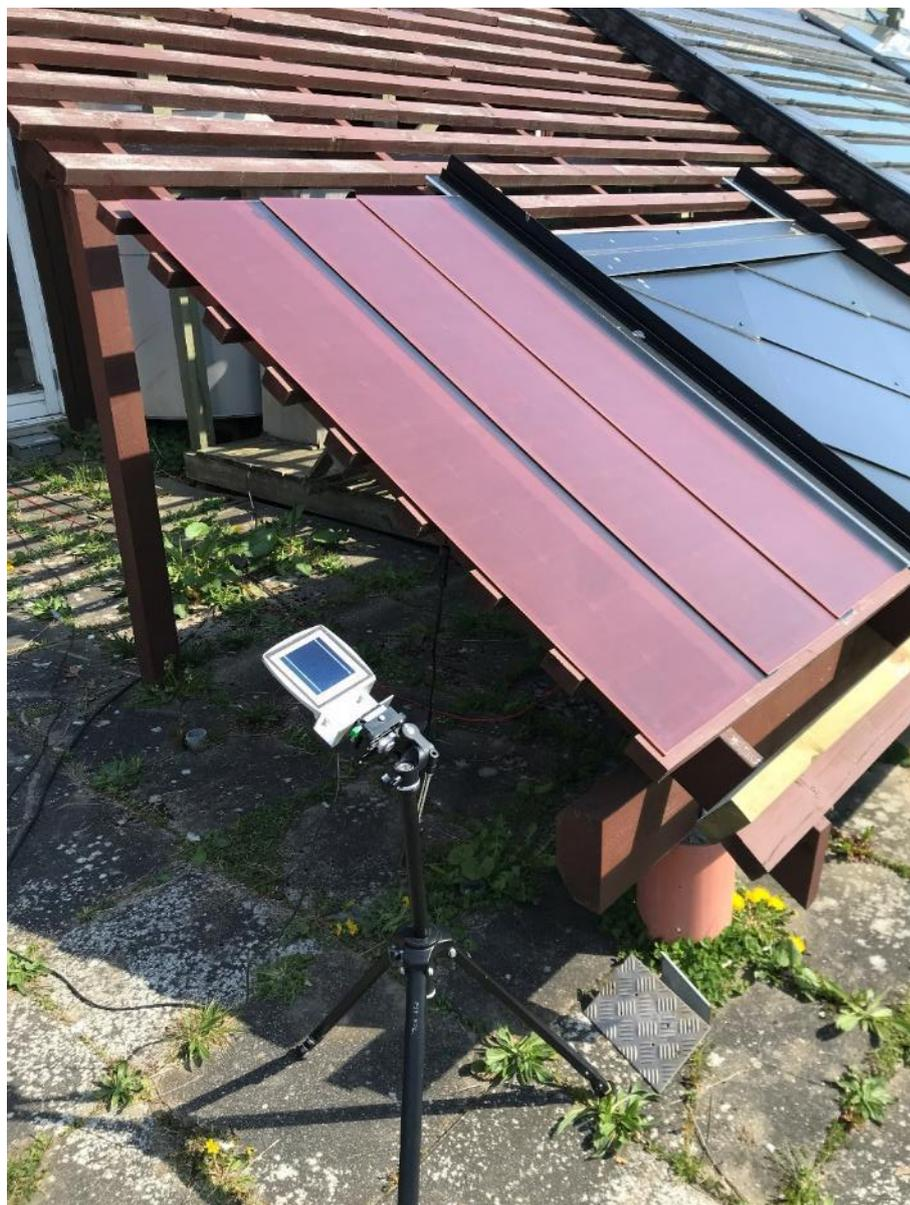
Figure 11 Set up for IV curve measurements with PVPM 6020 analyzer.
