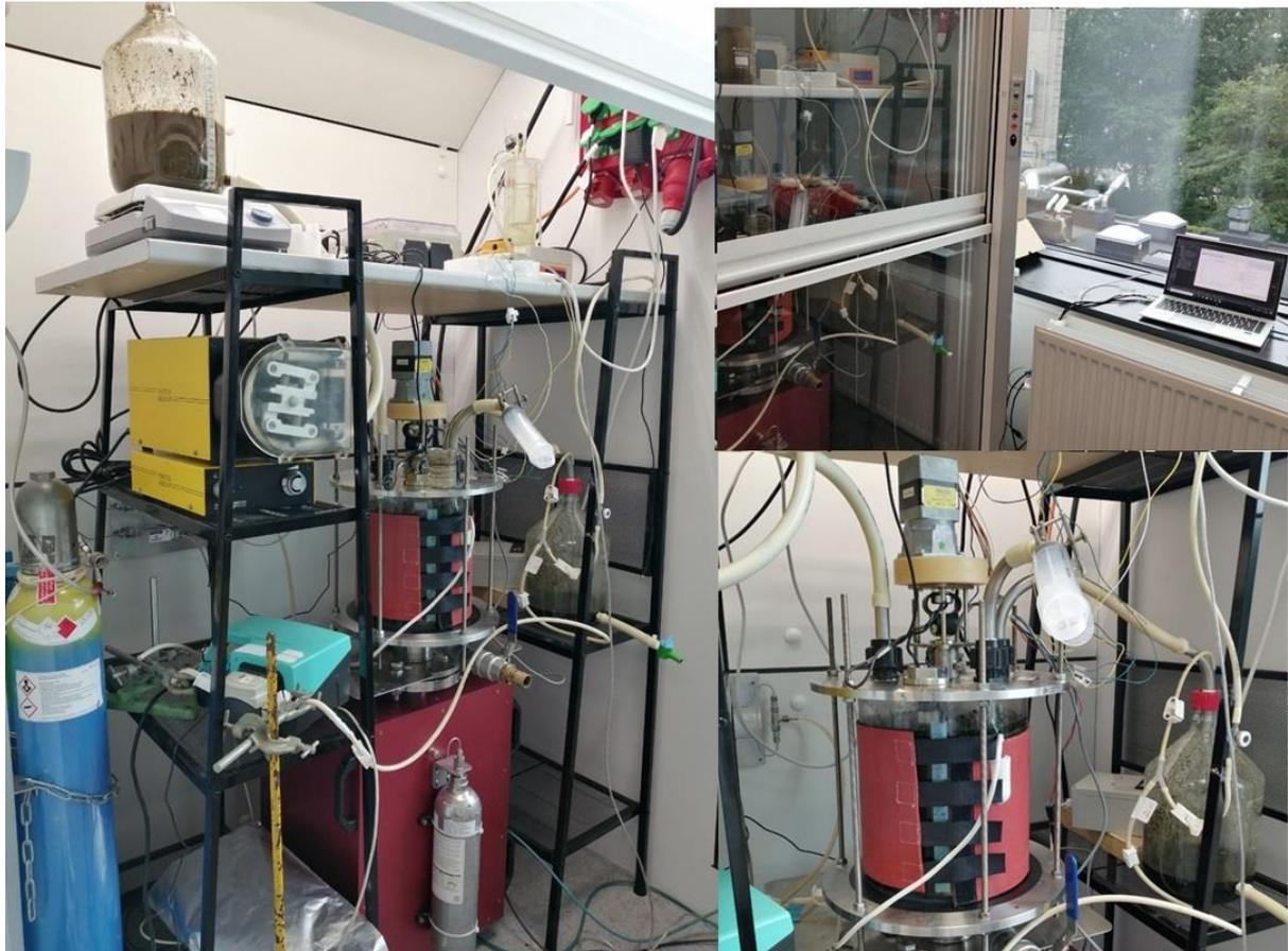
Figure 39 The final experimental set-up fed with cattle manure for biogas production.
