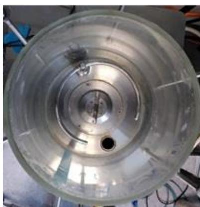
Figure 33 View from above of the installed gas sparger in the used reactor. In the center of the bottom of the reactor is visible the SPECTRO sensor
