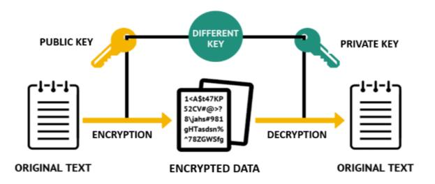
Using separate keys for encryption and decryption, as seen in the figure above, has helped eliminate key exchange, as seen in the case of symmetric encryption.
