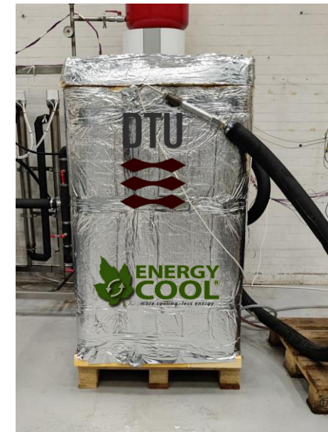
2 nd prototype: 230 L PCM
