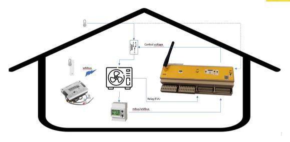
Figure 1: Hardware setup for PreHEAT Heat Pump Controller.
