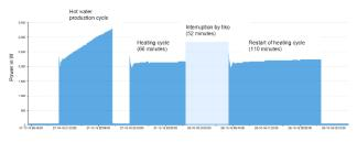
Figure 2: heat pump cycle interrupted by tiko control [1]
