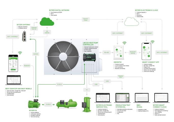
Figure 1: Overview of the Bitzer Heat Pump Ecosystem
