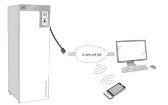
Figure 2: Representation of the interconnection between METRO THERM heat pumps and desktop through myUpway<sup>™</sup>.
