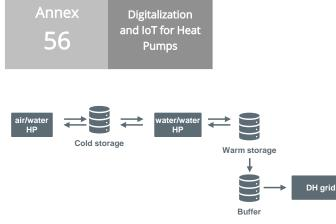
The concept ensures the use of excess electricity from the nearby wind park for heating purposes and provides therefore a unique flexibility option. This leads to significant reductions in:
