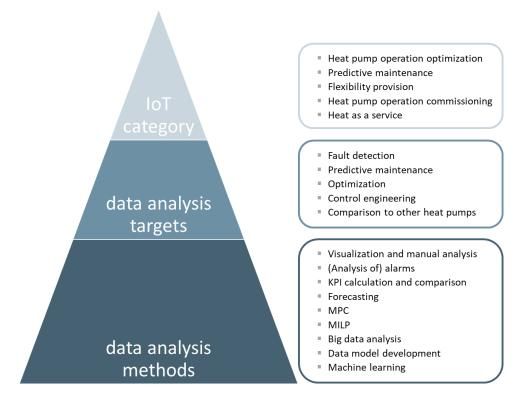
Figure 19: Hierarchy derived from the use cases: IoT category, data analysis targets and data analysis methods [9].
