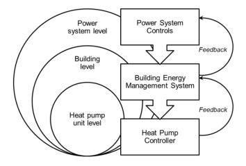
Figure 2: Control hierarchy and level of integration for heat pumps in smart grids [2].
