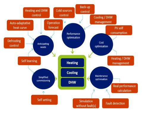
Figure 5: Use functions fulfilled by a heat pump.
