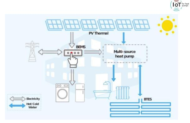
Figure 21. Concept overview for components in the RES4BUILD energy system.
