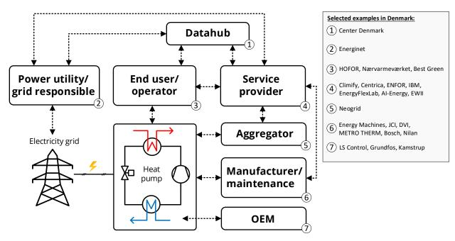
Figure 3. Visualization of supplier groups and examples of associated suppliers in an IoT-based energy system for heat pumps.
