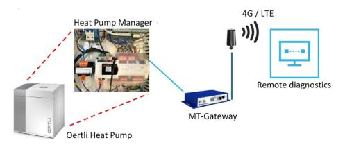
Figure 18: SmartGuard system setup [21].
