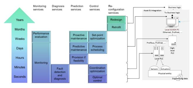
Figure 11: Categorization of services provided by digital twins according to scope, required response time and relevant system level on which the service is executed. The scope categories are based on [19].
