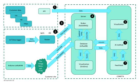
Figure 17: Data paths in the IoT based solution, made by Fraunhofer ISE [8].
