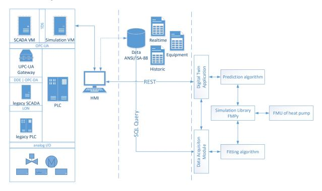
Figure 9: Functional and information structure of the DIGIBatch heat pump digital twin [8].
