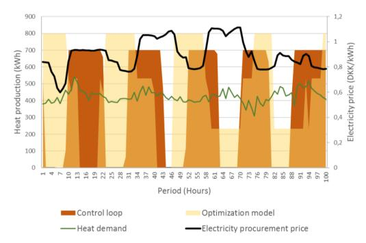
Figure 14. Flexible heat production during 100 hours period. "Control loop" with dark orange columns: Periods with heat production primarily from heat storage, and "Optimization model" with bright orange: Cost optimized heat production from heat pump (800 kW max. production). "Heat demand" is the heat demand in kW for the local district heating grid. Electricity price is seen on the y-axis on the right-hand side.
