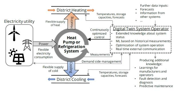
Figure 12. Diagram of the digital twin system operator.
