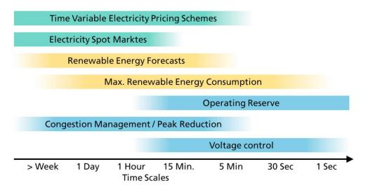
Figure 21: Time-wise characteristics of selected fields and mechanisms in the power system, where flexibility of the demand side might be used to create benefits [2].
