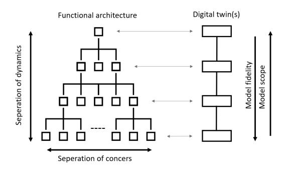
4.2.1.2.2 Functional architecture of a distributed digital twin
