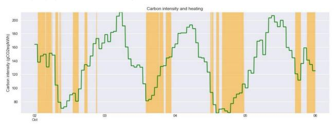
Figure 20. Predicted carbon intensity (green) and periods at which the heat pump is turned on (orange).
