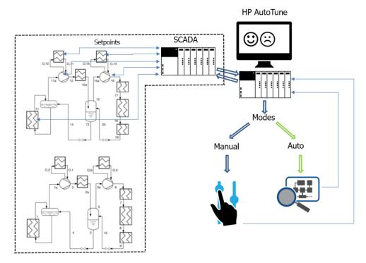
Figure 18. Concept for HP AutoTune.
