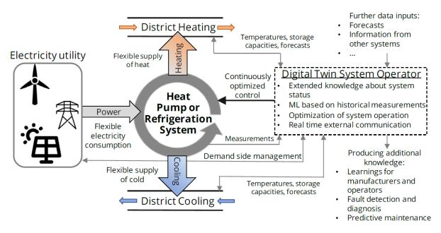
Figure 1: Diagram of the digital twin system operator.
