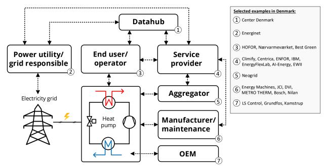
*Figure 24. Visualization of supplier groups and examples of associated suppliers in an IoT-based energy system for heat pumps.*
