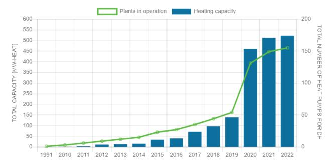
Figure 4. Overview of large-scale heat pumps for the Danish district heating network [13].
