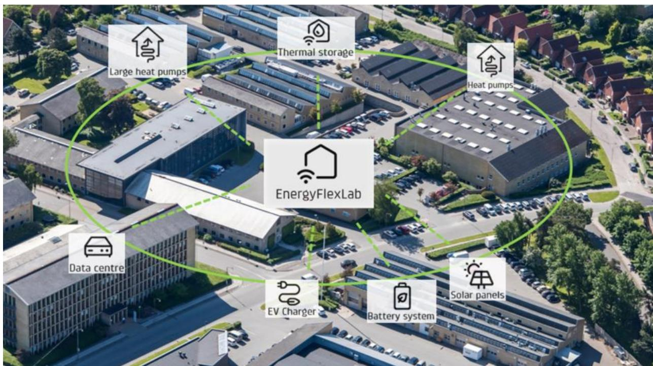
Figure 1: Main components in EnergyFlexLab.
